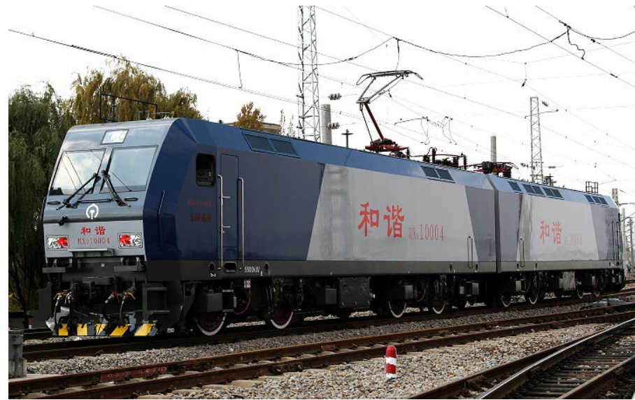
China Railway HXD1 series 12,900 hp freight locomotive set, under 25 kV overhead catenary wire pulls 20,000 ton coal trains
