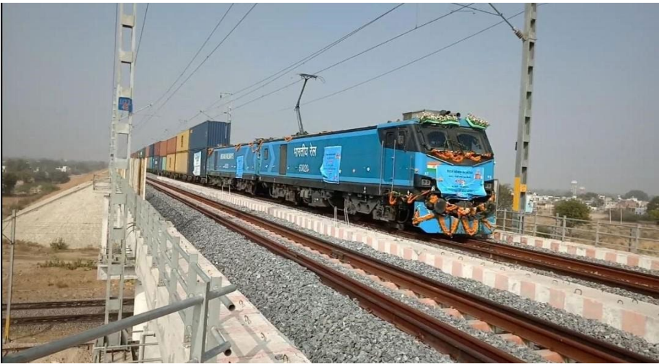
Electric train carrying double-stack containers under 25 kV wire in India
