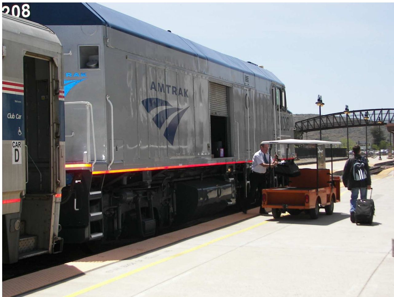
A converted F-40 as a combination Cab Car and Baggage Car or Cabbage Car seen here in 2008 in San Luis Obispo. These are usually used on low level push pull trains sets. Photo by Noel T. Braymer
